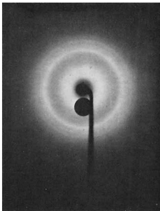
Fig. 6. Wide-angle x-ray scattering of U-51/PBA polyurethane.
